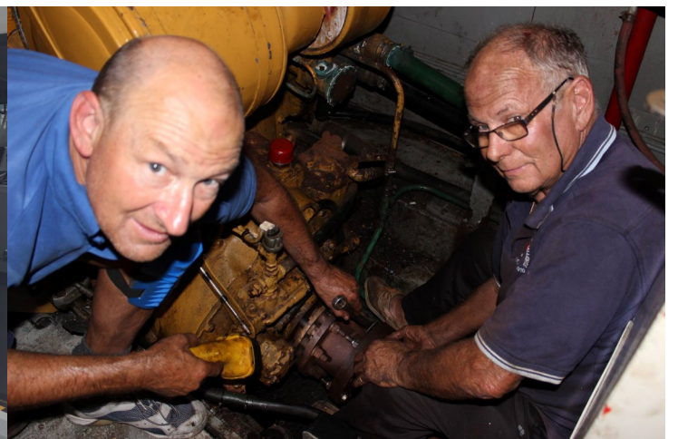
Bill and Robert working in very cramped and difficult conditions to drop back the shafts, they spent most of the day in that hole. Hot and dirty work in 2015.
