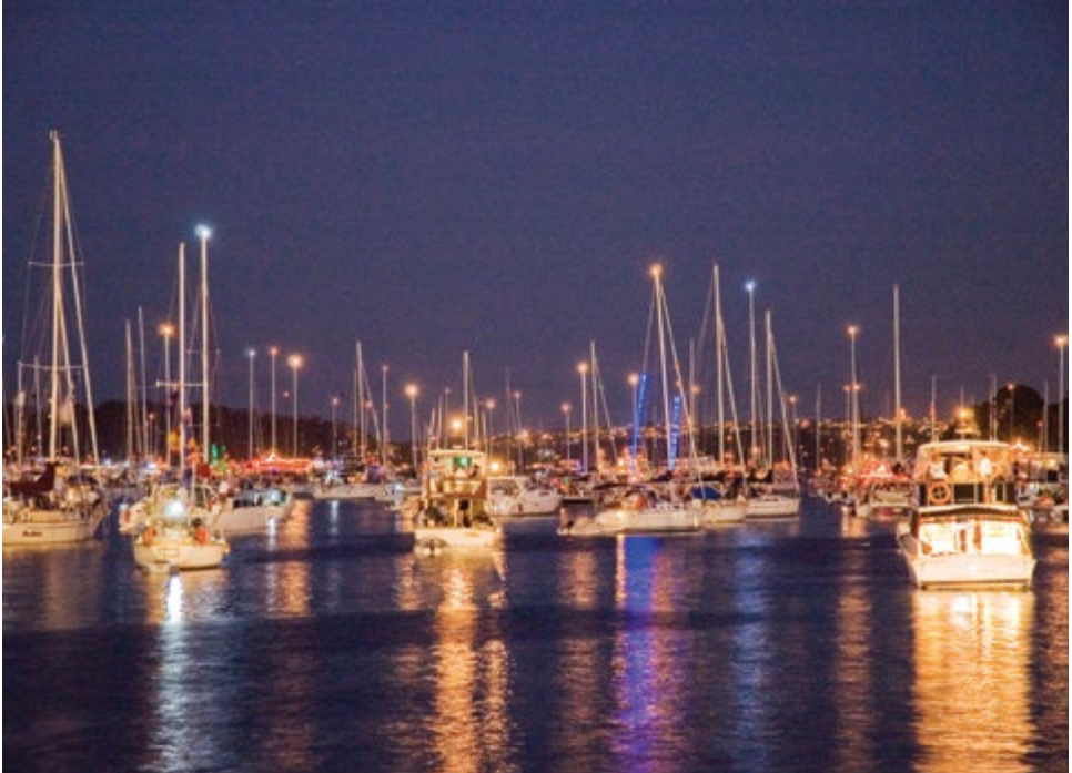
Vessels at anchor displaying all round white lights. Photo courtesy of City of Sydney.
