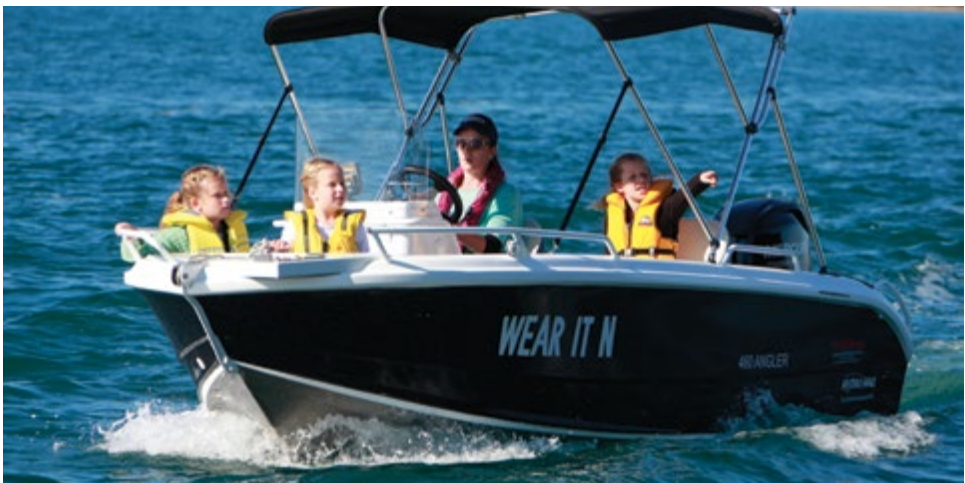
Vessel registration numbers/letters (in this case WEAR IT N) must be displayed on both sides of the hull.
